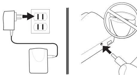
**WHEN TO RECHARGE** • Fully charge the power-pac before each use for best performance. The lithium ion battery in the power-pac will naturally discharge itself over time. It is best to charge it within two days of use. It is also recommended to fully charge the power-pac before storing it for extended periods of time. Store the power-pac in a dry, cool location – temperature no higher than 86°F (30°C).
